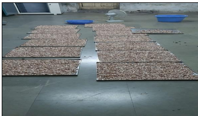
Fig.16 Output after drying 6hrs at 65 degree temperature maintained.
