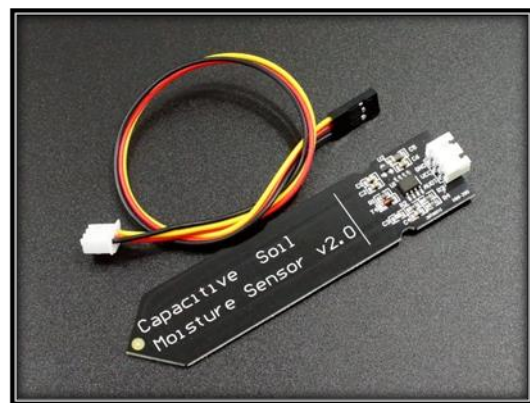
is specific lly m Fig.2. Capacitive Soil Moisture Sensor
