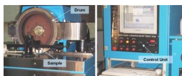
Fig1.schematic diagram of frictional material testing machine.
