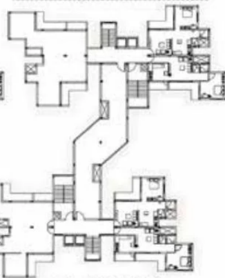
REFUGE FLOOR (AT 7TH FLOOR) AT SCALE 1:200
