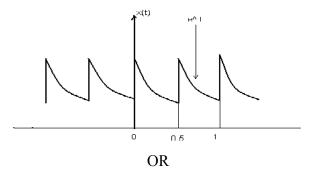
Qu2 A)Find trigonometric F.S. for the period signal x(t) shown in fig
