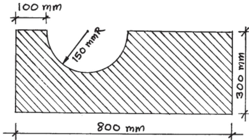
3. Locate the center of gravity for the solid as shown in Figure.
