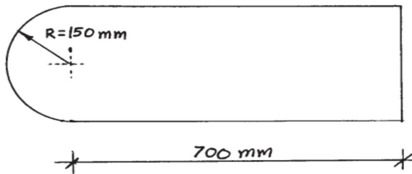
2. Locate the centroid of a shaded portion of a lamina as shown in Figure.
