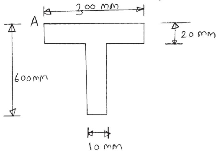
8. Calculate position of centroid of shaded area as shown in Figure.
