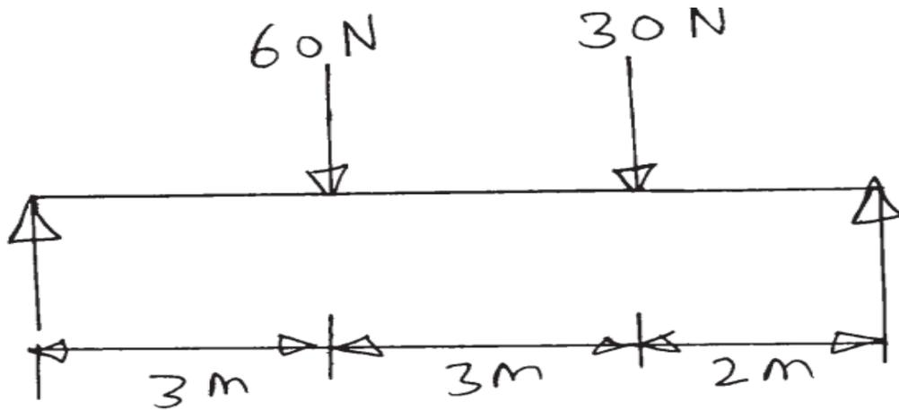
12. A simply supported beam of 6m span has subjected to loading as shown in Figure No. 4. Find support reactions by analytical method.
