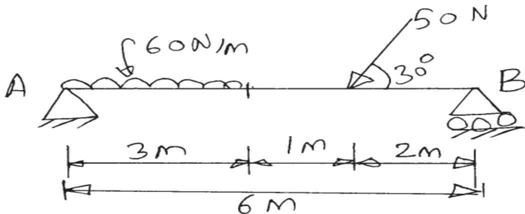
13. Calculate the reactions of beam loaded as shown in Figure No. 5 by analytical method.
