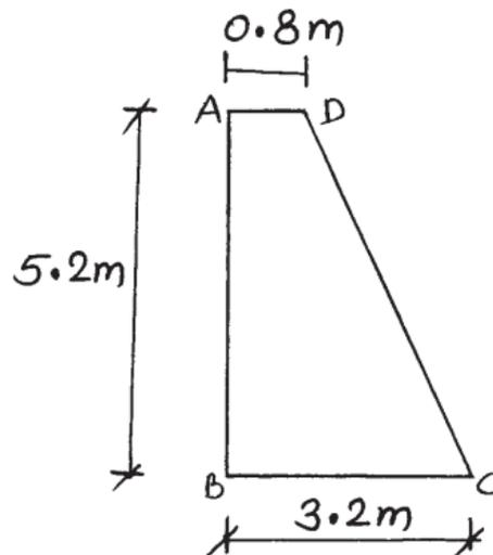
5. Locate the centroid of shaded area as shown in Fig.
