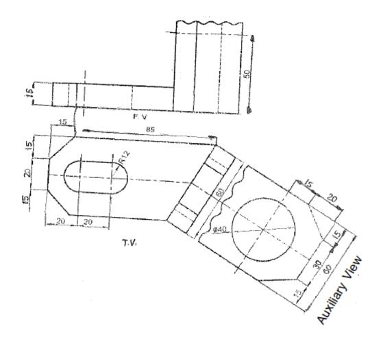
1. Figure shows incomplete top view, front view and auxiliary view. Draw the given views and complete the top view.
