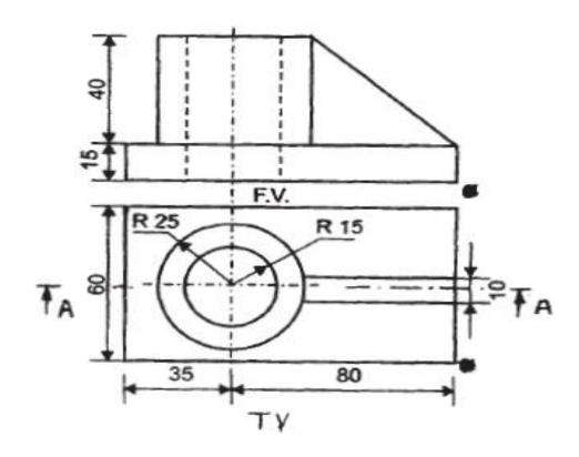
4. Figure shows incomplete front view, top view and auxiliary view of bracket. Draw the given views and complete the front view.
