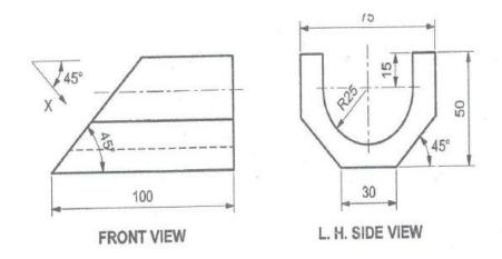
7. Figure shows front view and side view of object. Draw the given views and complete the auxiliary view.
