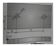
3) Write a program to mill slots of part as shown in fig. Make use of Subroutine. Plate thickness is 5 mm. Reference plane is 3 mm above the top surface. Cutter diameter is 5 mm. (CO5)
