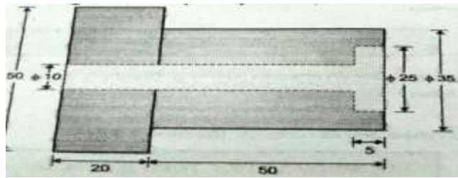
21. Prepare operation process sheet and sequence of operation for the ring nut assume suitable cutting parameter and raw material  $50 \times 10$ mm blank of carbon steel.
