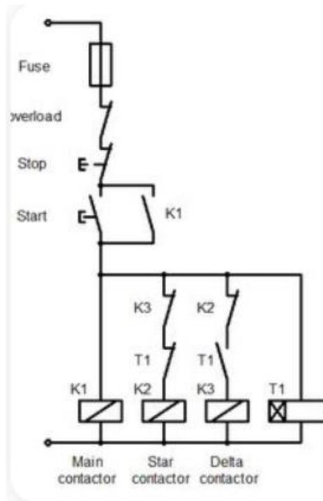
**Control Circuit diagram for star-delta starter**
