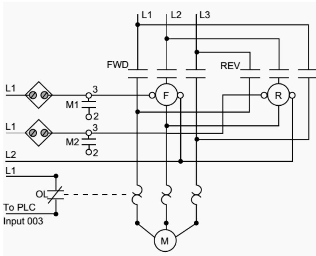
**Wiring Diagram of FOR-STOP-REV control of 3-phase Induction motor**
