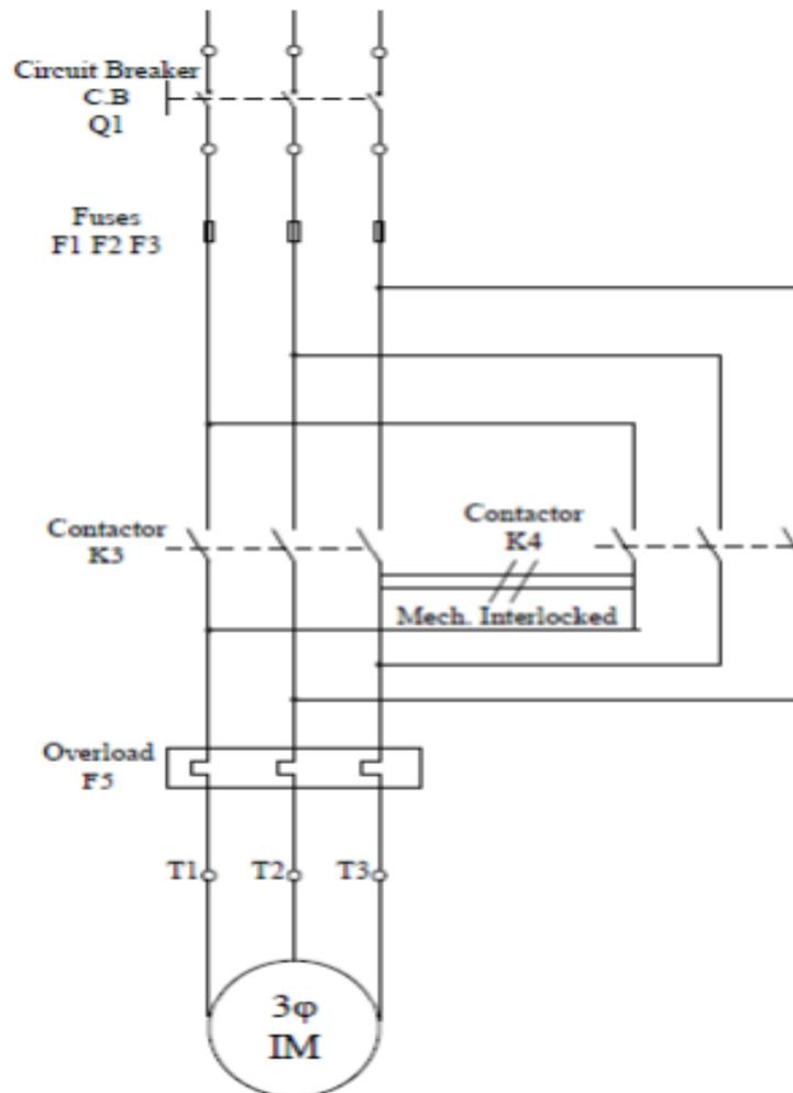
Reversing direction of rotation of a three phase induction motor, Power diagram
