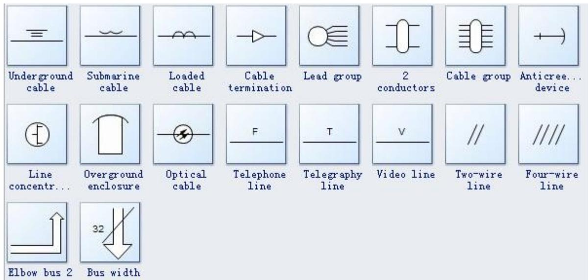
**Underground cable** is cable that is intended to be placed beneath the surface of the ground in ducts or conduit. Not necessarily intended for direct burial in the ground.
