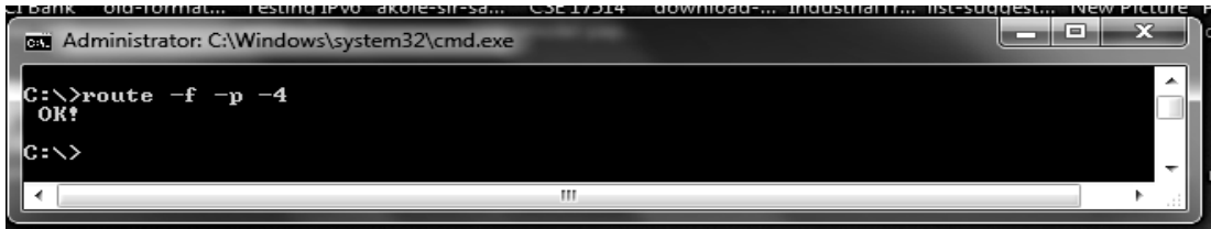
Fig. 10.1 : output screen of command c:\>route -f -p -4
