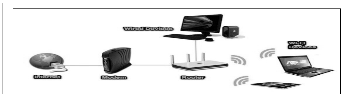
Fig. 11.4: Wireless Router connection diagram.
