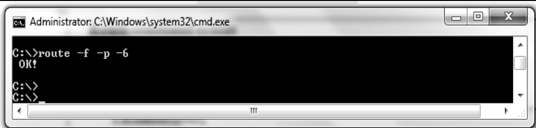
Fig. 10.2 : Output screen of command c:\>route -f -p -6
