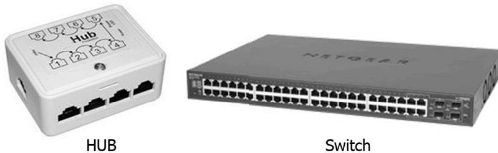
. Fig.7.1: Hub and Switch
