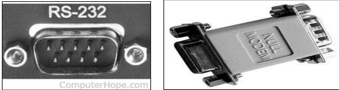
Fig 16.3: 9-pin RS-232 connectors and NULL MODEM Adaptor
